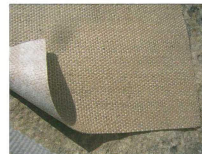
Fig. 2: Example of jute mat utilized in environmental restoration
